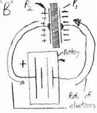
pressure of the battery and no current flows. The capacitor is now charged.
