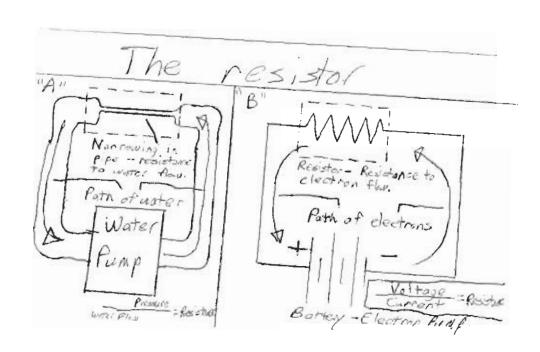
pressure is pushing a certain amount of water through the pipe system (per time unit). It seems reasonable that if we double the water pressure, the amount of water flowing through the system will also double (per time unit). It seems reasonable that the ratio pressure/amount of water flow will always remain the same, provided the resistance remains the same.
