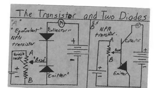
In "B" the same circuit as "A" is set up except the transistor equivalent is replaced by an actual transistor. We might expect to get the same results. We start with the variable resistor in position B. Sure enough, no current through meter M. We nudge the variable resistor toward A, but the current going through meter M goes way up! It only takes a very small base-emitter voltage to drive the collector current very high.
